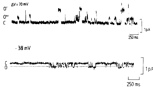
Fig. 1. Current fluctuations recorded from the plasma membrane of D. discoideum in the cell-attached mode. The upper trace shows two types of outward current ( O' and O'' ) fluctuations obtained at 70 mV depolarization ascribed to the channel types DI and DII resp. The lower trace shows inward current fluctuations ascribed to channel HI obtained from a different cell at a 38 mV hyperpolarization. Recording conditions were: 15 mM NaCl, 1 mM KCl, 2 mM \text{CaCl}_2 , pH 6.9, stage t_5 (upper trace) and 15 mM KCl, 2 mM \text{CaCl}_2 , pH 7.0, stage t_{6.5} (lower trace).
